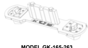
MODEL GK-165-263 Consists of two (2) GK-165-211 magnets with on/off switch in a self aligning support bar assembly. Track datum height 3-1/8" (79.4 mm)
